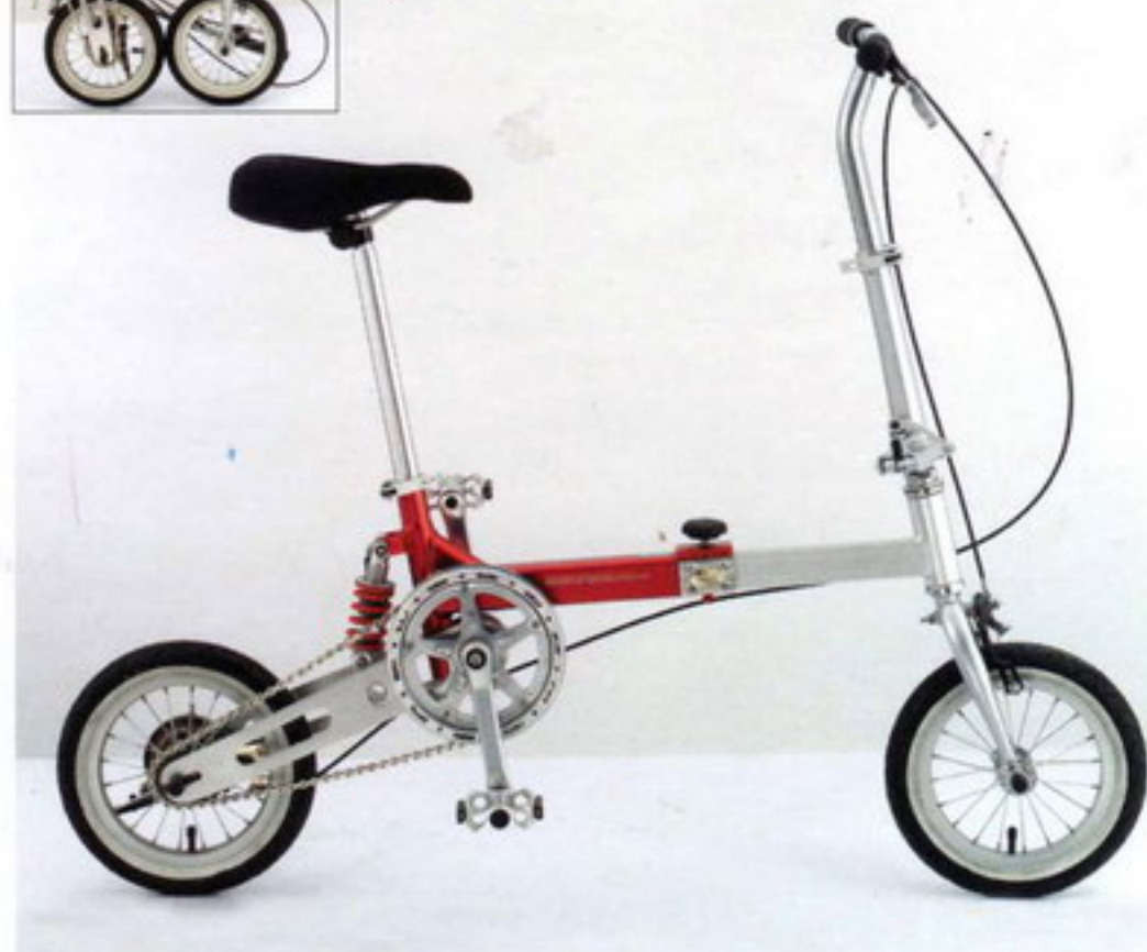
Model: YHC-FD-1233-A ALUMINUM FRAME FC LENGTH ADJUSTABLE TO SUIT INDIVIDUAL NEEDS OFFERS EASE OF STORAGE
