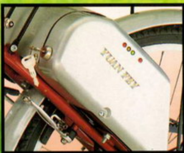
BATTERY POWER INDICATION LAMP
